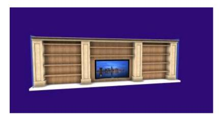
This unit is 161 ½ inches wide and 50 inches tall. It will be installed on a 46 inch shelf in the family room. There are four columns. The two outside columns meet flush with the surrounding walls. The two middle columns have molding wrapped on three sides at the bottom. The shelves will sit on shelf pegs mounted in ¼ inch holes on the columns. The spacing of the holes is yet to be specified.
